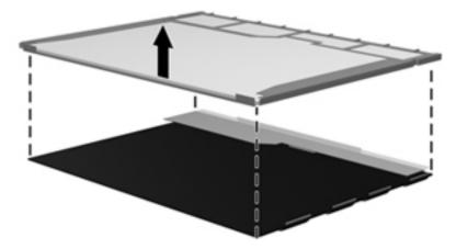
**24.** Recycle the LCD panel and backlight.
